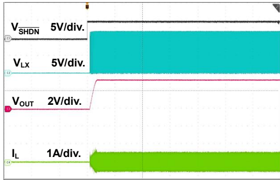
Figure 16. Startup Through \overline{SHDN} Waveform
