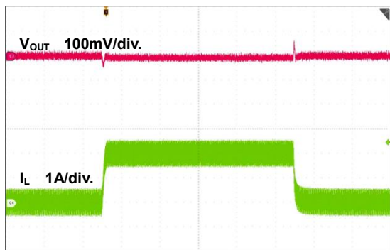
Figure 20. Load Transient Waveform
