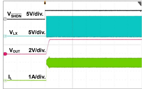
Figure 17. Startup Through \overline{SHDN} Waveform
